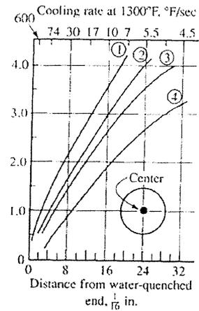
Relationships between cooling rates in round bars and in Jominy locations. (1 = still water; 2 = mildly agitated oil; 3 = still oil; 4 = mildly agitated molten salt).
