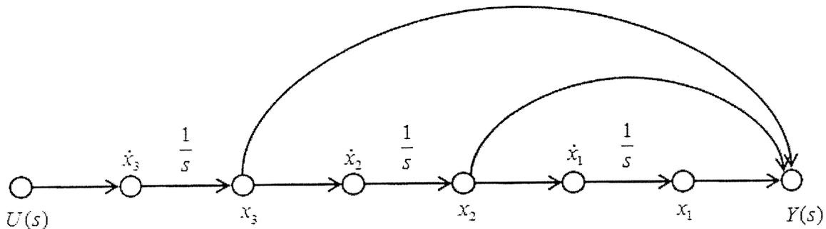
**Figure Q8.1** – Complete the Signal Flow Graph Representing  $G(s)$
