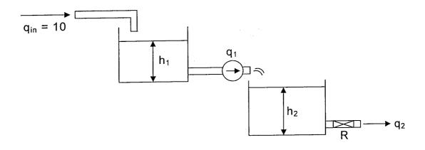
Two tanks are connected in series in a noninteracting fashion as shown in the figure.
