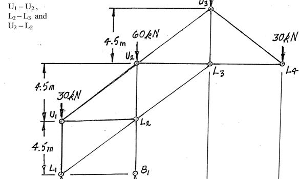
(18) 5. For the frame shown below, using the moment-distribution method or the slope-deflection method, calculate and plot the shear force and bending moment diagrams. On both diagrams, for each member, label the maximum and minimum ordinates. (Minimum ordinates are frequently negative values.) All members have the same EI value and are inextensible.
