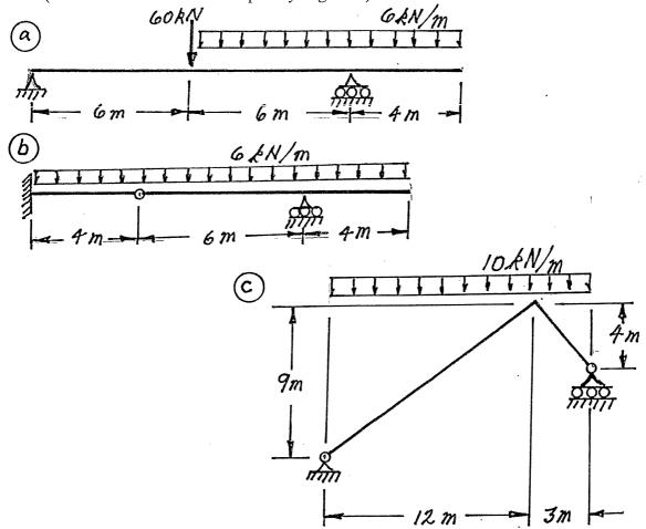
(18) 3. Calculate the vertical deflection at point  $\bigcirc$  on the continuous beam shown below. EI = 2000 kN.m<sup>2</sup> for all beam segments. Take advantage of symmetry.
