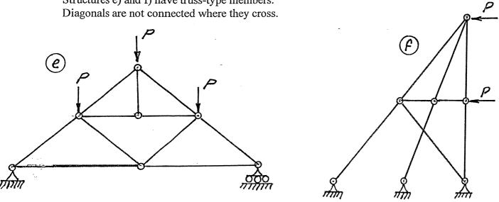
(18) 2. For each structure shown, compute the reactions and draw shear and bending moment diagrams. Indicate which are positive and which are negative segments of each bending moment diagram. For each member on the shear and bending moment diagrams, calculate and indicate the magnitudes of the maximum and minimum ordinates (Minimum ordinates are frequently negative.).
