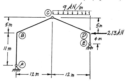
Using the principle of virtual work, calculate the horizontal deflection at point  $\bigcirc$  of the structure shown below. The tie rod has an AE = 4.5 x 10<sup>4</sup> kN. Both beams are inextensible and have EI =  $2.4 \times 10^5 \text{ kN.m}^2$ .
