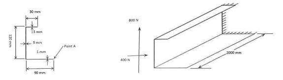
Q4. Idealize the box section shown here to direct stress carrying booms at four corners and shear stress carrying panels.
