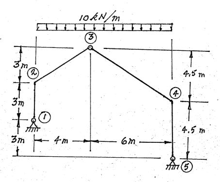
Use the principle of virtual work to obtain the vertical deflection at point of the beam shown below. EI is constant and equal to 1.7 x 10<sup>3</sup> kN.m<sup>2</sup>.
