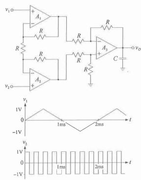
Given that all the op amps are ideal. The power supplies for op amps are  $\pm 15$ V.
