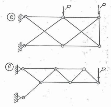
(18) 2. For each structure shown, compute the reactions and draw shear and bending moment diagrams. Indicate which are positive and which are negative segments of each bending moment diagram. For each shear and bending moment diagram, calculate and indicate the magnitudes of the maximum and minimum ordinates (Minimum ordinates are frequently negative values).
