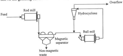
After grinding in a rod mill, the ore is sent to a magnetic separator to remove the non-magnetic wastes before being fed to the ball mill. The following operating data are available:
