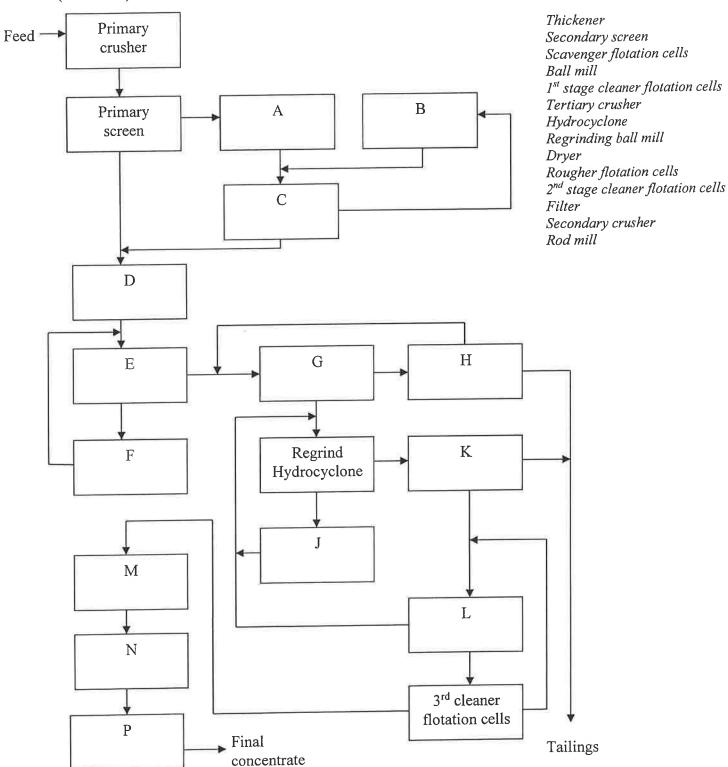
The following shows the grinding circuit for an iron ore.
