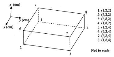
(a) [4 marks] Determine the shape functions  $(N_i, i = 1 \text{ to } 8)$  of an eight-node hexahedron element in natural/local coordinates  $(\xi, \eta, \zeta)$  such that  $-1 \le \xi, \eta, \zeta \le 1$ . The node numbering is identical to that shown in the above representative global element.
