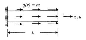
$$EA\frac{d^2u(x)}{dx^2} + cx = 0 \quad 0 < x < L \qquad subject to: \quad u(0) = 0 \quad and \quad EA\frac{du(x)}{dx}\bigg|_{x=L} = 0$$
