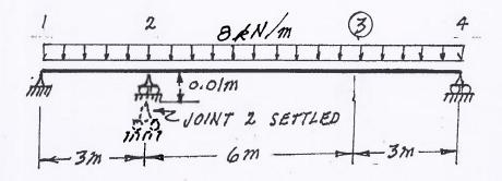
Using the slope-defection method or the moment-distribution method, analyse the structure shown below. Plot shear force and bending moment diagrams. On each diagram for each member, label the maximum and minimum ordinates (Minimum ordinates are frequently negative values). All members are inextensible and have the relative EI values shown on the structure.
