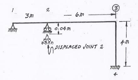
Use Castigliano's theorem (the "least work" theorem) to analyse the two-beam structure shown. Calculate and plot the shear force and bending moment diagrams for both beams. On each diagram, calculate and label the maximum and minimum ordinates (Minimum ordinates are frequently negative values). Both beams are inextensible and have the same EI value.
