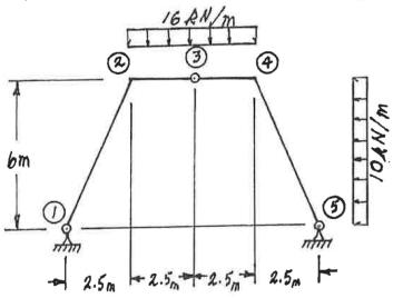
Use the **principle of virtual work** to calculate the horizontal deflection at joint 2 on the frame shown. All members are inextensible and have  $EI = 1.8 \times 10^5 \text{ kN.m}^2$ .
