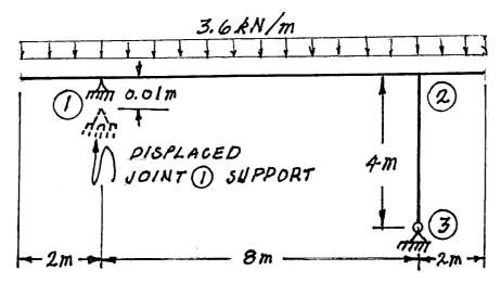
Using the slope-defection method, analyze the structure shown. Draw shear force and bending moment diagrams. On each diagram, for each member, calculate and label the magnitudes of the maximum and minimum ordinates (Minimum ordinates are frequently negative values). All members have the same EI value and are inextensible.
