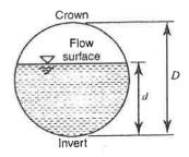
Nomenclature: d = partial depth D = full depth or pipe diameter q = partial discharge Q = full-flow discharge v = velocity, partially fullV = velocity, full
