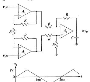
Given that all the op amps are ideal. The op amps' power supply is  $\pm 15$ V. Also, R = 10k $\Omega$  and C = 10µF.
