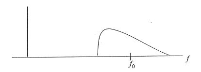
a) Give the block diagram of a system that transforms the above signal to a bandpass signal with the same carrier frequency but with a spectrum that is the mirror image about the carrier frequency (for positive frequencies), i.e. the spectrum is as follows (for positive frequencies).
