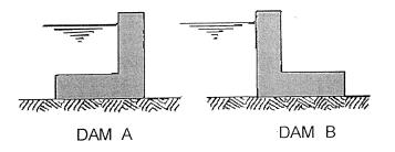
Two small L-shaped dams are built on a firm flat surface as shown above. Assuming that there is no seepage under the wall but that sliding can occur, state which dam - Dam A or Dam B - will be most likely to slide. Explain fully why one will be more likely to slide than the other.
