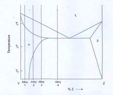
(c) Which of the alloys (1,2,3, and/or 4) in the figure above could be strengthened by age hardening? (Assume that β forms a coherent precipitate in α). Outline the complete procedure for the age hardening process.
