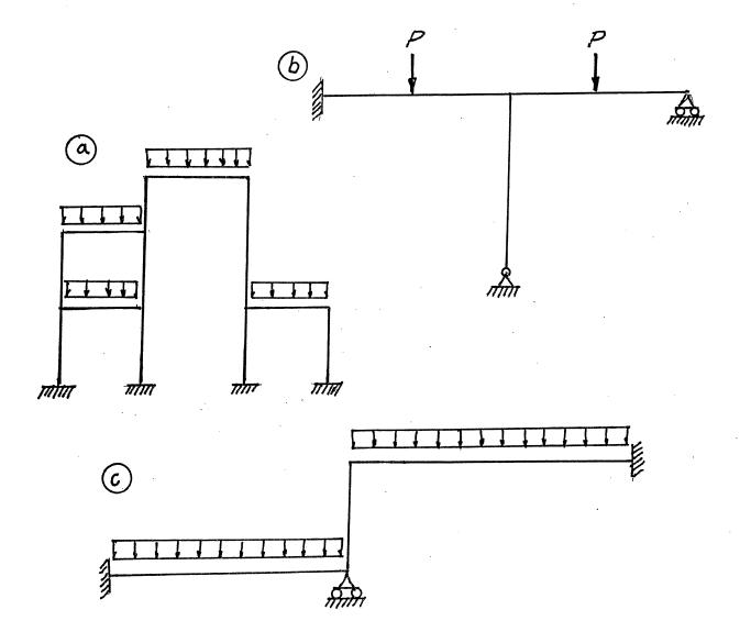
(12) 2. Schematically show the shear force and bending moment diagrams for the following structures. All members have the same EI and are inextensible.
