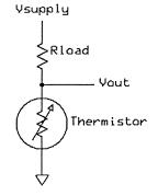
c)(3 marks) Why should the load resistor be chosen to equal the resistance of the thermistor in the middle of the expected temperature measurement range?
