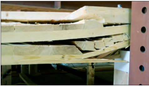
Point-supported cross-laminated timber panel testing apparatus and failure
