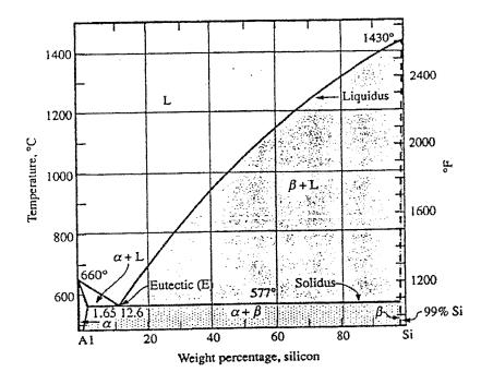
Fig 3. Aluminum – Silicon Phase Diagram
