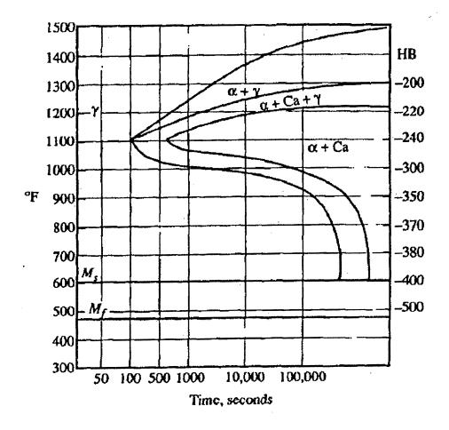
Fig 2. Temperature Time Transition Diagram for 1035 carbon steel
