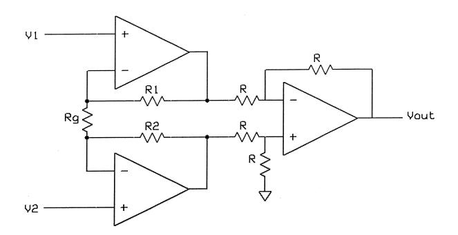
The schematic diagram describes a typical instrumentation amplifier.
